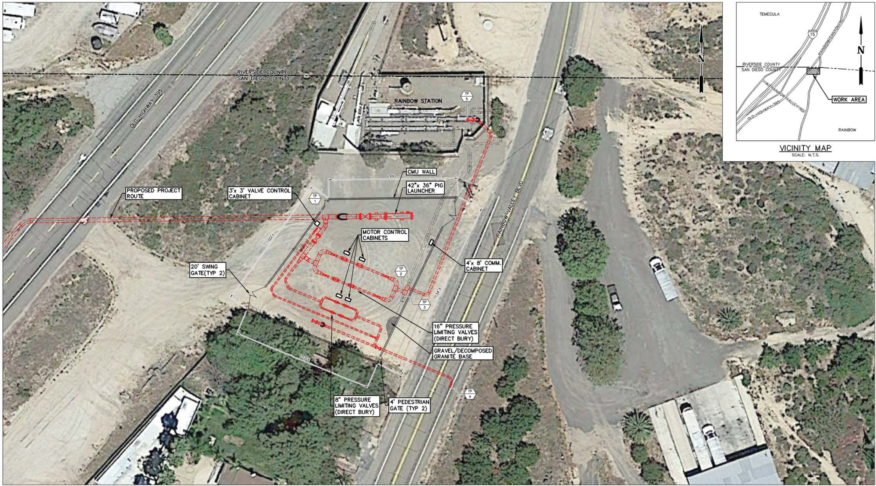
Figure 2.2-1: Rainbow Pressure-Limiting Station Site Plan
